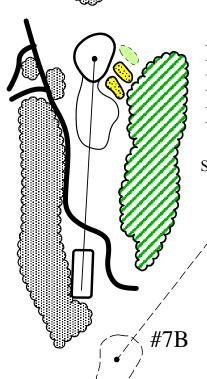
Remove Sand Bunker (1,157 sf) Rebuild Sand Bunker (1,173 sf) Rebuild Sand Bunker (987 sf)
